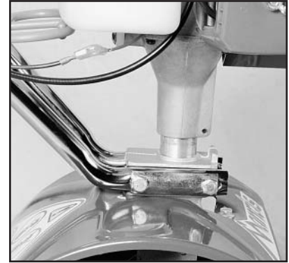
Picture 1 ... Note how the engine doesn't sit all the way down on the transmission.
