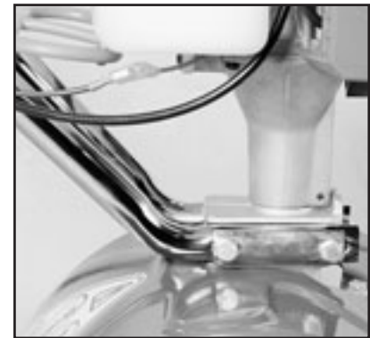
Picture 2 ... Note how the engine sits all the way down on the transmission.
