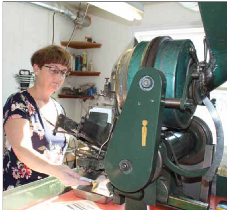
Pauline Hager operating a circa-1950s seed packaging machine, still very much in use today at Veseys. Seeds are dropped into a hopper and a predetermined quantity is fed into the packets. Replacement parts for the machine must be made from scratch, as they are no longer manufactured. (Nicole Kitchener photos)
